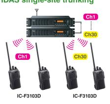
The IC-F3103D series can be used in an IDAS single-site trunking system.
