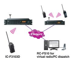
When using the IC-F3103D series in IDAS multi-site conventional mode, the IC-F3103D can communicate with other IDAS radio users working with other repeater sites and/or virtual radio/PC dispatch stations on the IDAS network.
