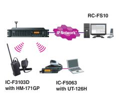
When used with the optional GPS speakermicrophone, HM-171GP, GPS position data can be sent to other advanced IDAS radios (PC and software required) and/or virtual radio/PC dispatch stations.
